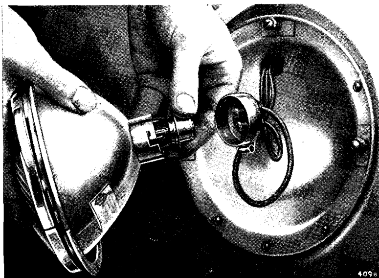
Fig. 20. Head lamp light unit with backshell removed.
